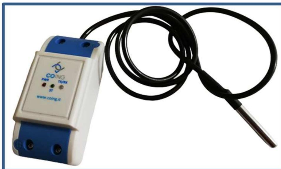
**DISPOSITIVO EMBEDDED BASATO SU TECNOLOGIA "LoRa" PER IL MONITORAGGIO DELLA TEMPERATURA DA SONDA ESTERNA**
